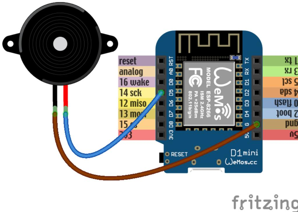
The piezoelectric speaker doesn't use any external source of power – it will be powered directly from the GPIO pin – that's why it can be pretty quiet. Still, let's try it:
