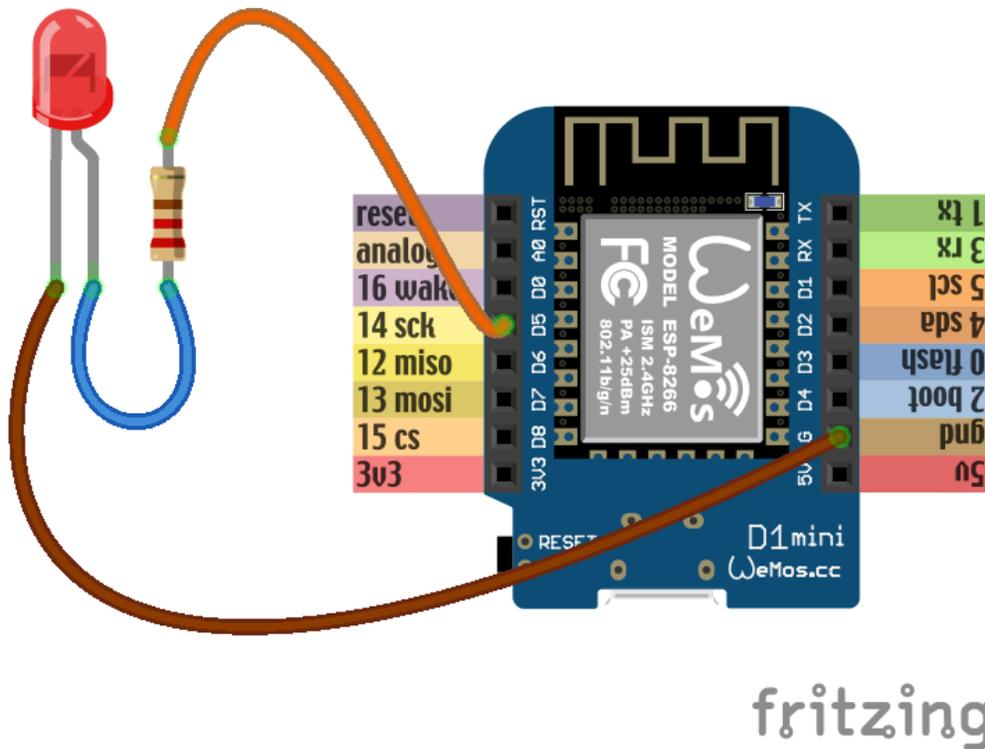
Note how one leg of the LED is a little bit longer, and the other had a flattening on the plastic of the LED next to it. The long leg should go to the plus, and the short one to the minus. We are connecting the LED in opposite way than the internal one is connected – between the pin and gnd. That means that it will shine when the pin is high, and be dark when it's low.
